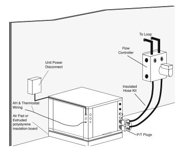
**NOTICE!** Cabinet opening around loop piping (outdoor compressor section) must be sealed to prevent entry of rodents that could potentially damage unit wiring by chewing on the insulation.
